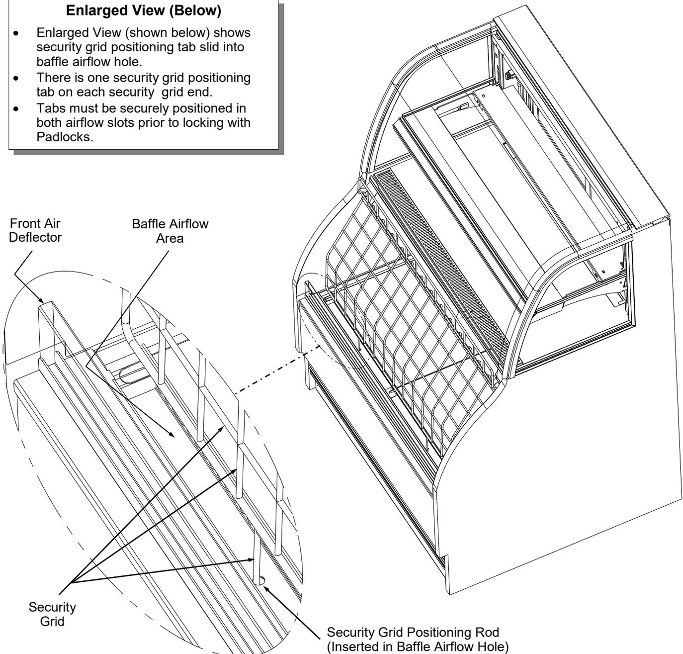
**Securing Security Grid Into Place and Locking**
