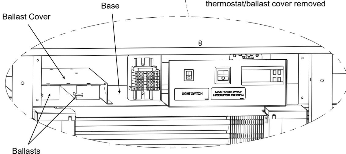
Enlarged view of thermostat/ballast area
