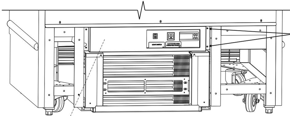
Remove two (2) screws at each end of cover to remove thermostat/ballast cover.
