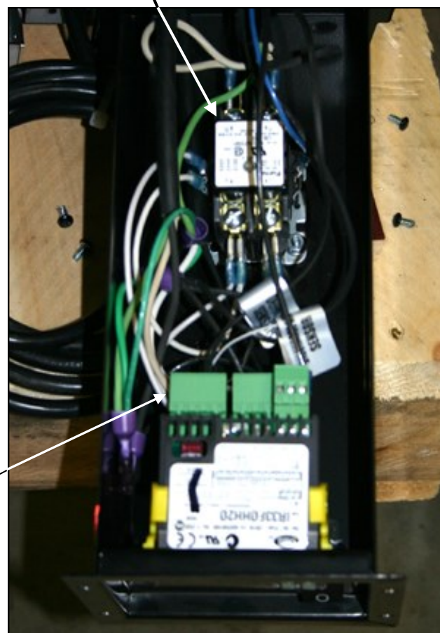
Top View of LED Controller in LED Controller Box
