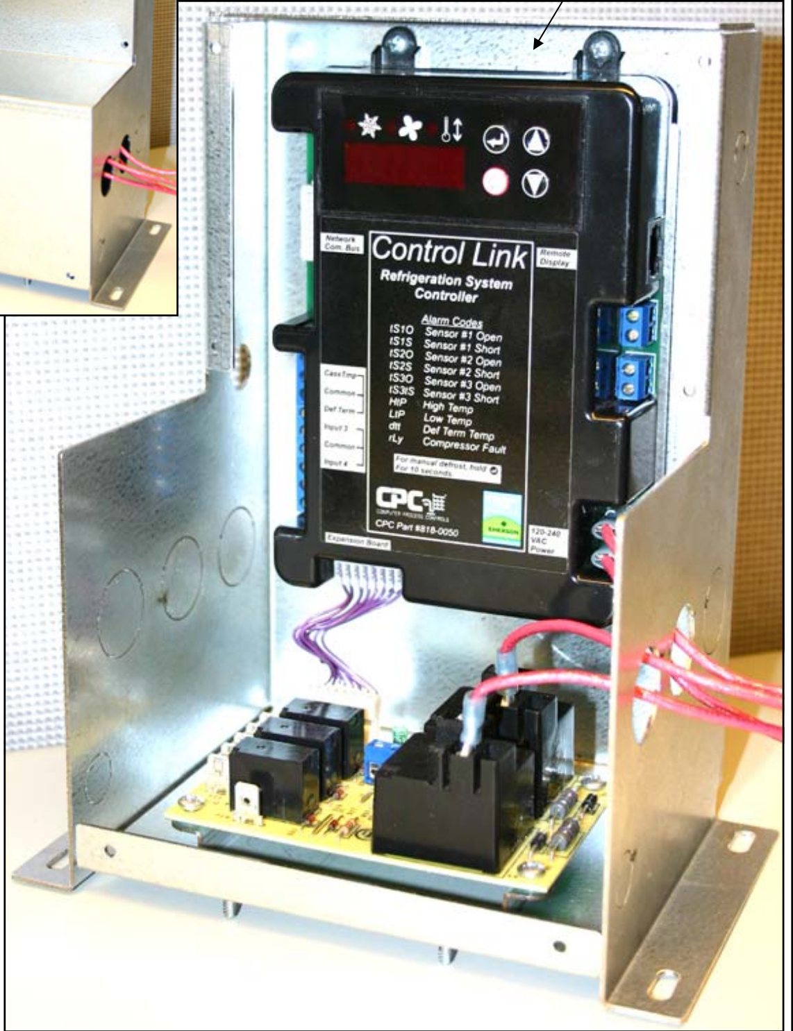
View of Control Link Refrigeration System Controller With Housing Cover Removed
